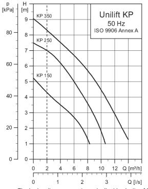
The broken line represents a min. liquid velocity of 0.7 m/s with a DN 32 discharge pipe to DIN EN 12056.
