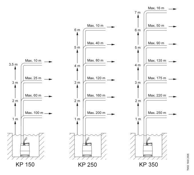
The above overview is only intended as a guide. Grundfos is not liable for any faulty installations based on the overview. **Note:** If the non-return valve is used, the pressure drop in the valve is 0.2 m head, which is to be subtracted from the vertical pipe lengths.
